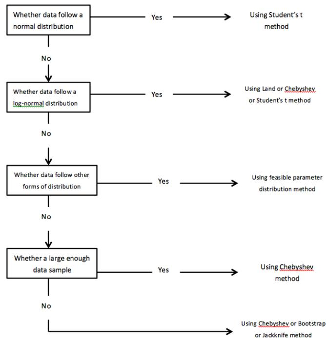
**Figure 1. Flowchart Tocalculate UCL Value**
