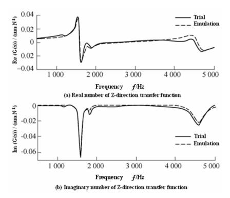
Figure 8. Transfer Function of Mill's Knifepoint in z Direction
