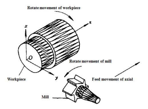
Figure 1. Mainly Movements in Orthogonal 4-axial Turn-Milling
