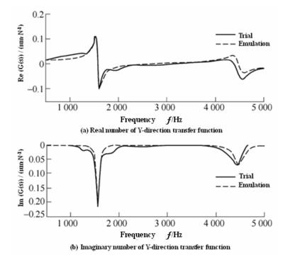
Figure 7. Transfer Function of Mill's Knifepoint in y Direction
