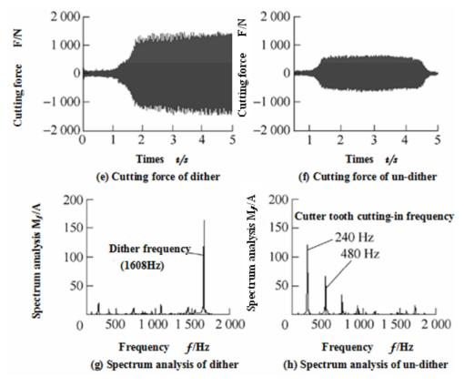
Figure 9. The Stable Range Leaf Figure of Dither and Results of Analysis in 4-axial Turn-Milling
