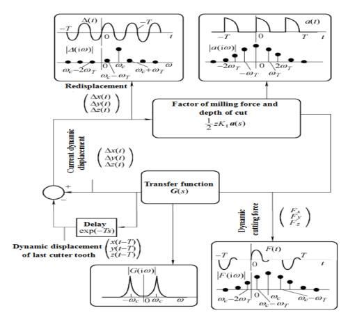
Figure 3. The Regenerative Dither in Turn-Milling by End Mill during Machining
