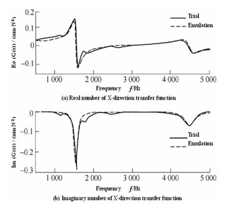
Figure 6. Transfer Function of Mill's Knifepoint in x Direction
