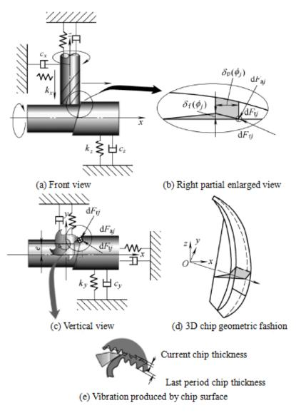
Figure 2. The 3d Shape of Chip when End Mill and Workpiece Vibrating Relatively in Three Direction
