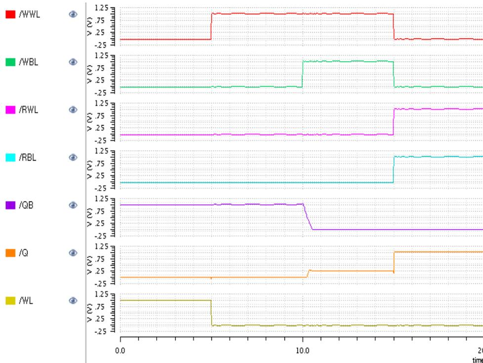
**Figure 4. Waveform of the Operation Held in Proposed 8T SRAM Bit Cell**
