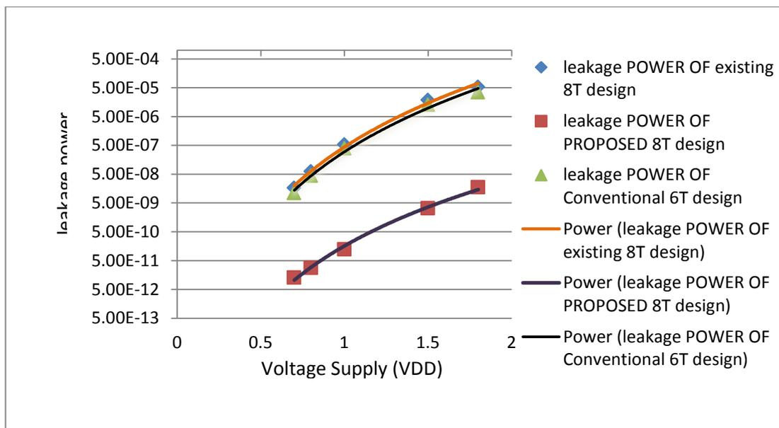
**Figure 5. Comparison between Standby Leakage Power of Conventional 6T, Existing 8T and Proposed 8T design at 45nm CMOS Technology**
