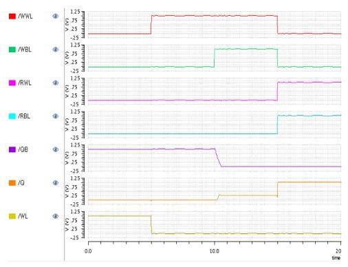
Figure 4. Waveform of the Operation Held in Proposed 8T SRAM Bit Cell
