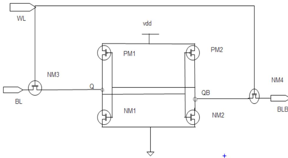
**Figure 1. Schematic of conventional 6T SRAM bit – cell**
