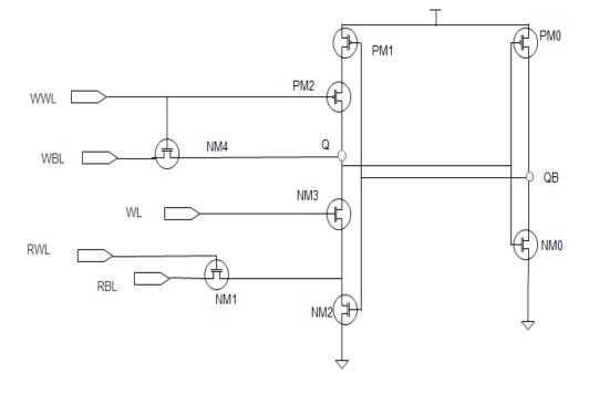
Figure 2. Schematic of existing 8T SRAM bit – cell
