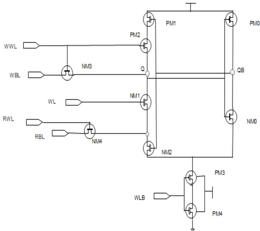
**Figure 3. Schematic of Proposed Asynchronous Single Ended 8T SRAM bit – cell**
