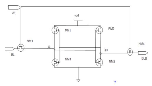
Figure 1. Schematic of conventional 6T SRAM bit – cell
