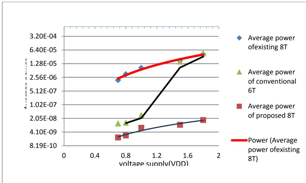
**Figure 8. Comparison between Average power of conventional 6T, existing 8T and proposed 8T design at 45nm CMOS technology**
