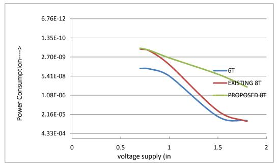
Figure 6. Write '1' Active Power at Different Voltage Supply of Different Memory Cells
