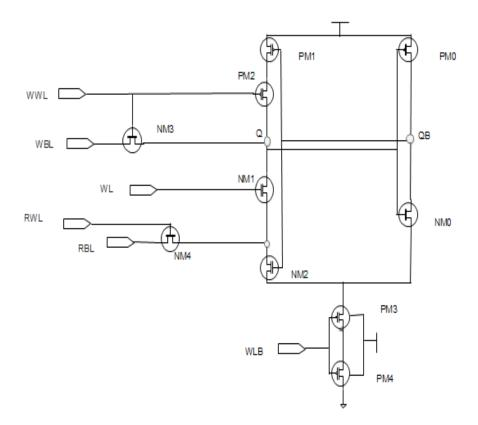
Figure 3. Schematic of Proposed Asynchonous Single Ended 8T SRAM bit – cell
