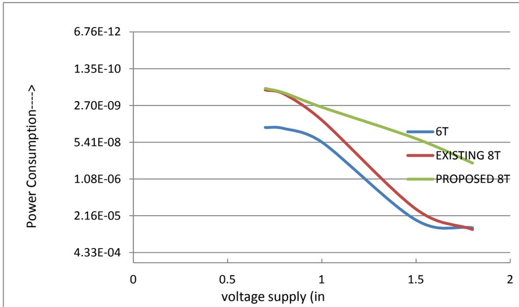
**Figure 6. Write '1' Active Power at Different Voltage Supply of Different Memory Cells**
