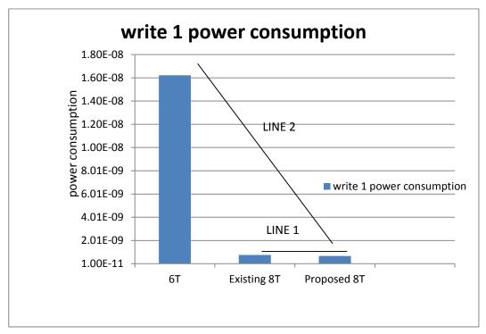
Figure 7. Write '1' active power consumption in the different memory cells at 0.7volt power supply
