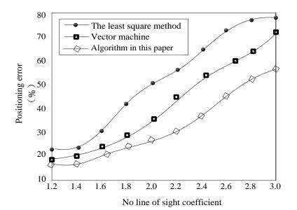
Figure 4. Relationship between Non-Light-of-Sight Coefficient and Three Algorithms' Positioning Errors
