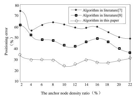
Figure 2 Influence of Anchor Density on Three Algorithms' Positioning Accuracy
