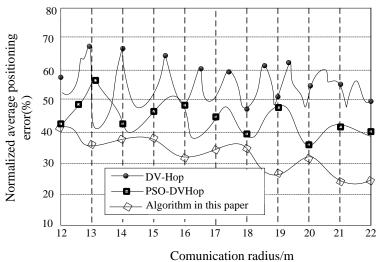
Figure 6. Positioning Performance of the Three Algorithms under Different Communication Radius
