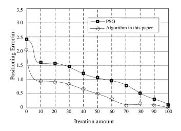
Figure 3. The Position Error Variation Curve of this Paper Algorithm and PSO Algorithm
