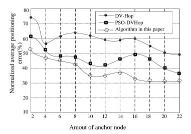
Figure 5. Positioning Performance of Three Algorithms with Different Number of Anchor Nodes
