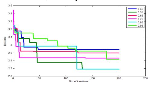
Figure 2. Analysis of Convergence Pattern for Varied Inertia Weight Value
