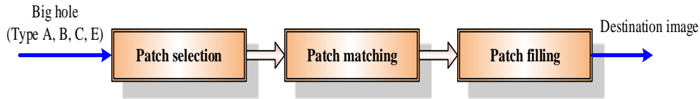
Figure 6. Flowchart of the Improved Exemplar-based Inpainting Algorithm
