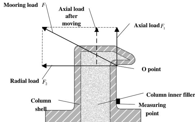
**Figure 3. Bollard Structure and Force Analysis**
