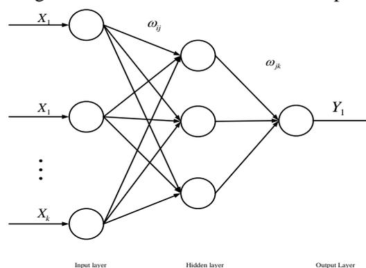
Figure 1. The Topology Diagram of BP Neural Networks
