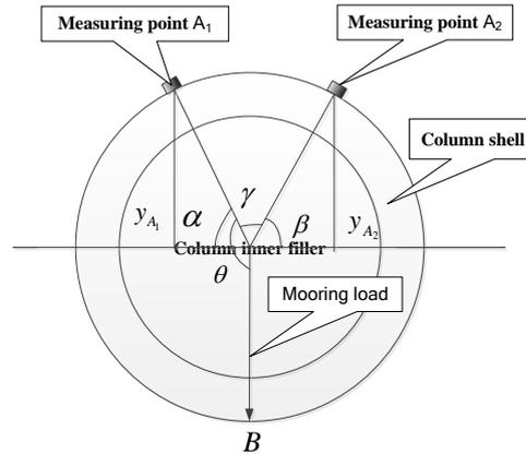
**Figure 4. The Distance between Each Measuring Point and the Neutral Axis**
