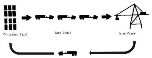
Figure 1. Illustration of the Integrated QC-YT Operation
