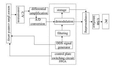
Figure 1. ECT Data Acquisition System
