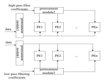
Figure 6. Filter Based On Double Multiplier
