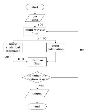
Figure 2. Flow of Wavelet Kalman Algorithm
