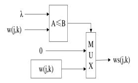
**Figure 7. Hard Threshold Function**
