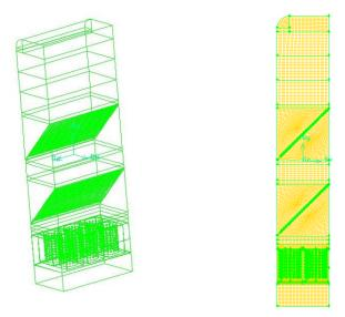
Figure 2. Geometry Modeling and Grid Division
