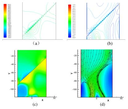
Figure 5. Pressure and Velocity Distribution Of Needle Plate-Type Low-Temperature Plasma Generator
