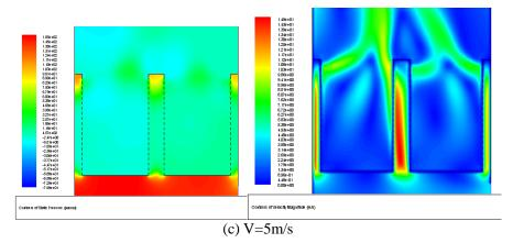
Figure 4. Pressure & Velocity Distribution in the Primary Filtering Cartridge
