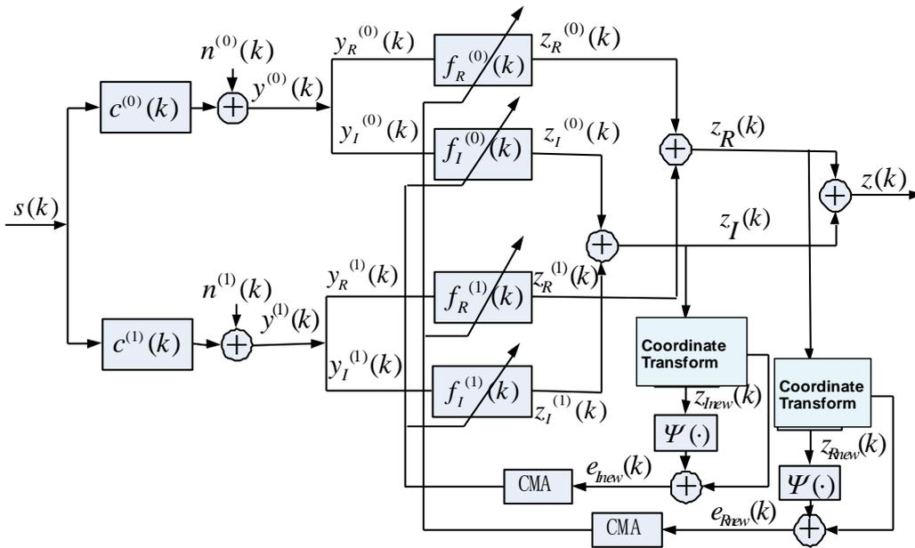
**Figure 2. An Improved T/2 Fractionally Spaced Blind Equalization Algorithm with Coordinate Transform**
