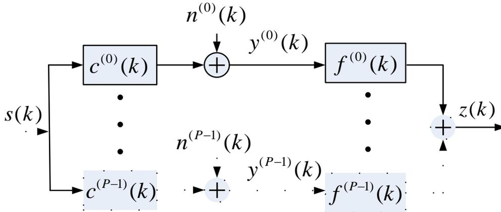
**Figure 1. Structure of Fractionally Spaced Blind Equalizer**
