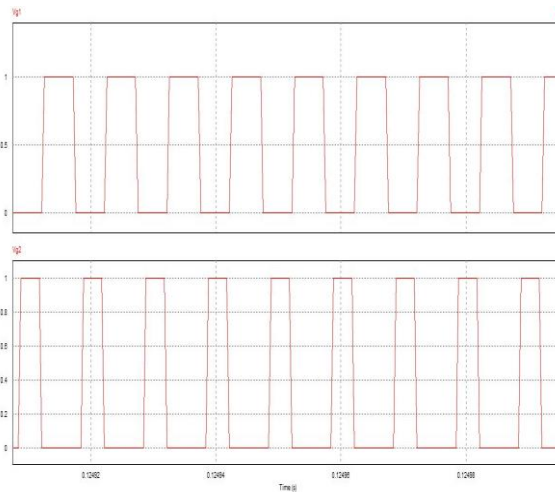
Figure 7. Gate Control Waveform of the switches S1 and S2
