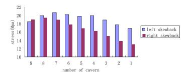
Figure 7. Comparison between Left Skewback and Right Skewback About Stress
