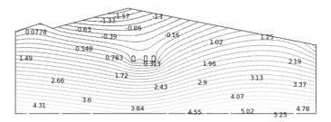
Figure 10. Pore Water Pressure after Excavating the Left 3 Tunnels
