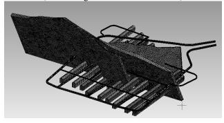
Figure 3. Finite Element Mesh for Caverns
