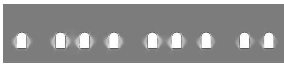
Figure 8. Equivalent Plastic Strain around the Caverns
