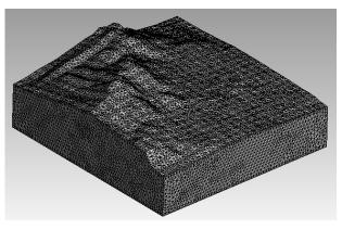
Figure 2. Finite Element Mesh for Rock Mass
