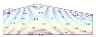
Figure 9. Water Pressure Contour Map before Excavation (Mpa)
