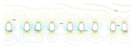
Figure 5. Contour Map for Vertical Direction after Excavation
