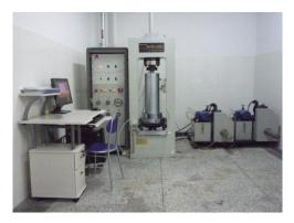
Figure 1. RLW-500 Rock Triaxial Apparatus for the Test
