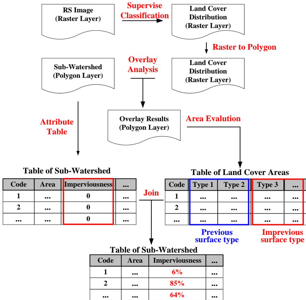
**Figure 4. The Processes of Imperviousness Collection for Each Sub-Watershed Based on GIS**
