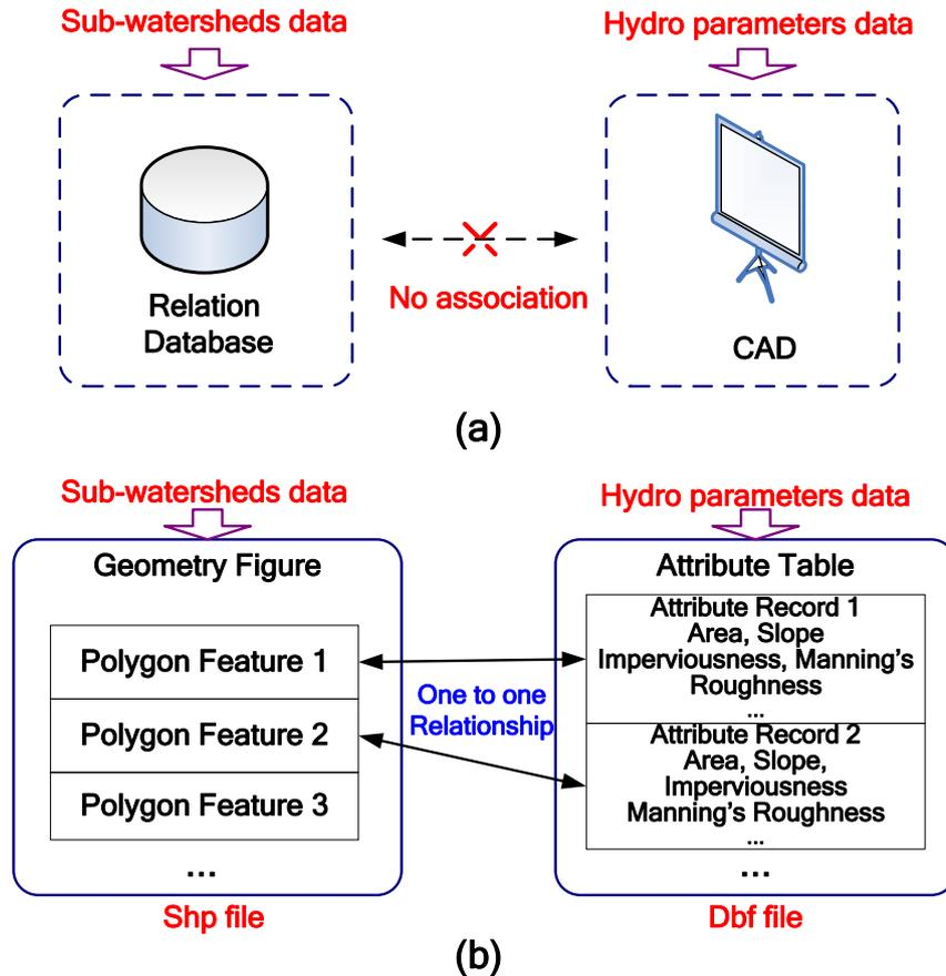
**Figure 1. Data Storing Structure of the Sub-watersheds and Hydrological Parameters. (a) Traditional Method. (b) GIS-based Method**
