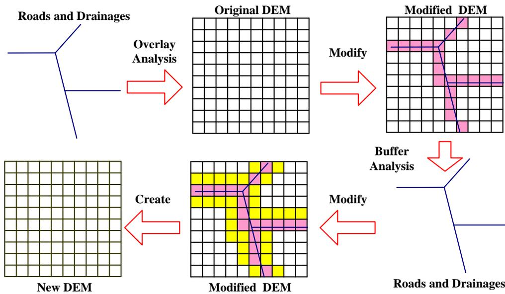
**Figure 3. Information Processing of the DEM Data by Using the Spatial Analysis in GIS**
