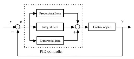
Figure 2.1. PID Control System Structure Diagram
