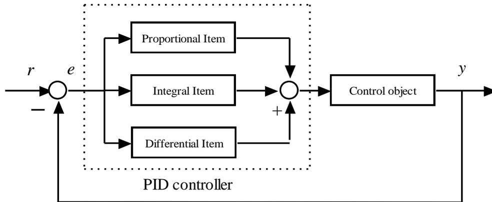
Figure 2.1. PID Control System Structure Diagram
