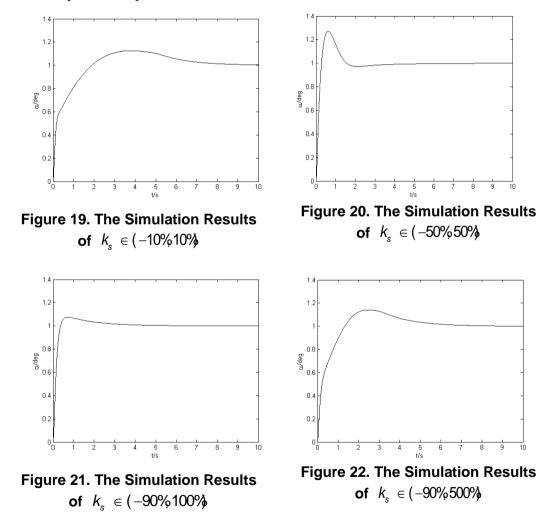
The simulation results are stable under the condition of different perturbation. It shows that the control method has strong robustness.
