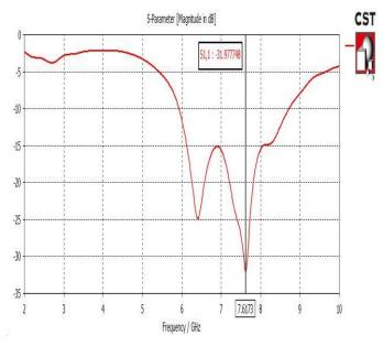
Figure 9. Return Loss of Brain Phantom Model with Miniaturized UWB Antenna Is 31.97db at 7.6173 Ghz
