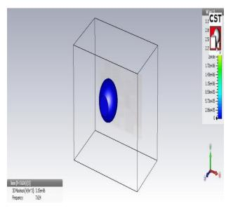
Figure 11. SAR of Miniaturized UWB Antenna with Brain Model Is 3.15\*10<sup>6</sup>
