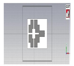
Figure 2. Front View of UWB Planner Antenna
