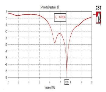
Figure. 4. Return Loss of the UWB Planner Antenna 45.76 db at 7.624 Ghz
