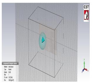
Figure 12. Perspective View of the Brain Phantom Model with Triangular Tumor at Center of the UWB Antenna
