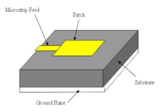
Figure 1. Rectangular Microstrip Patch Antenna
