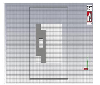
Figure 3. Modified Ground Plane of the UWB Planner Antenna
