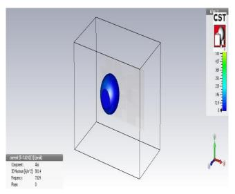
Figure 10. Current Density of Miniaturized UWB RMPA with Brain Phantom Model Is 801.4A/m<sup>2</sup>
