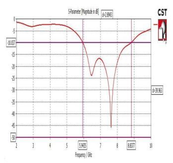
Figure 5. Bandwidth of the Planner UWB Antenna Is 2.8493 Ghz
