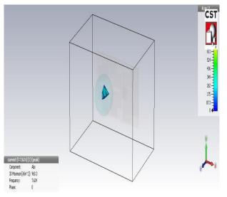
Figure 14. Current Density of Miniaturized UWB Antenna with Tumor in the Center of the Brain Is 960.3A/m<sup>2</sup>
