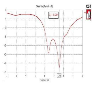
Figure 13. Return Loss of Brain Phantom Model with Cancer Tumor in the Center Is 32.52db
