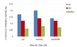
Figure 2. The Specific Unbalance of Different Resource by Three Algorithms
