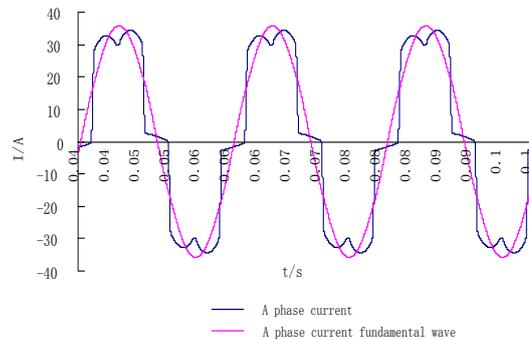
Figure 8. Phase a Current Fundamental and Harmonic Compared
