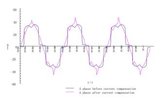
Figure 10. Phase a Current before and After APF
