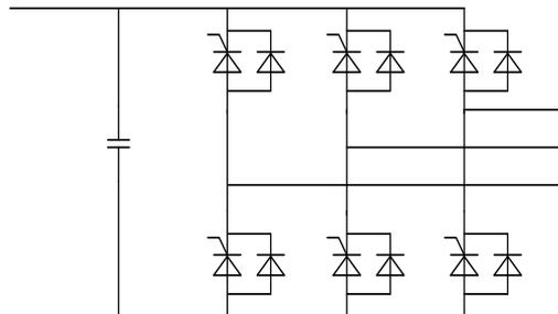
**Figure 3. Device Structure of Reactive and DC Bias Compensation**
