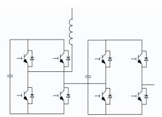
Figure 2. Configuration Diagram of Multi-Stage Inverter
