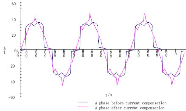
**Figure 10. Phase a Current before and After APF**
