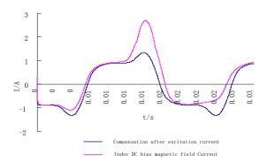
Figure 12. Excitation Current Waveform Before and After DC Bias Compensation
