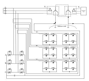
Figure 4. Overall Topology of the Compensation Device
