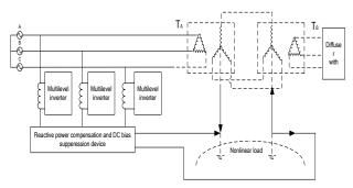
Figure 1. Schematic of Comprehensive Compensation Device
