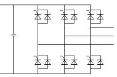
Figure 3. Device Structure of Reactive and DC Bias Compensation
