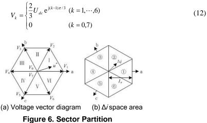
Eight switch states corresponding to the APF output voltage vector are in the area of a hexagon. The area is divided into six symmetrical triangles, as shown in Figure 6 (a). In order to reduce the difficulty of discriminating the positive and negative polarity of  $\Delta i_a$ ,  $\Delta i_b$  and  $\Delta i_c$ ,  $\Delta i$  space area is divided into six triangle area, noted as (1-6) hysteresis width is  $I_w$ , as shown in Figure 6(b).
