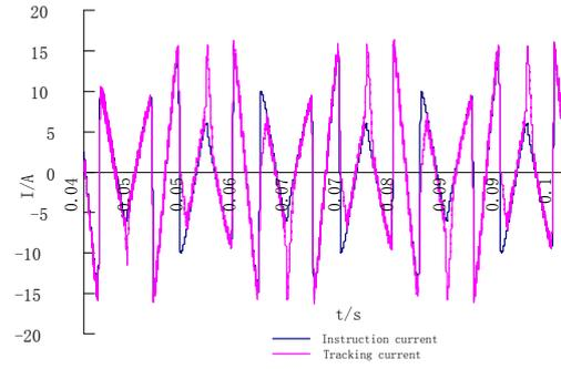
**Figure 9. APF Instruction Current and Tracking Current**
