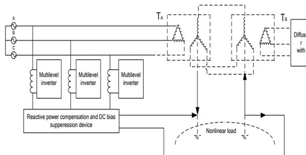
**Figure 1. Schematic of Comprehensive Compensation Device**
