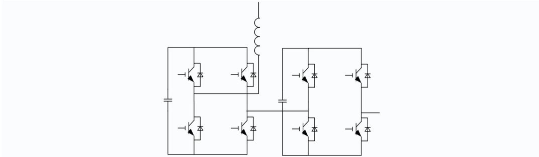
**Figure 2. Configuration Diagram of Multi-Stage Inverter**
