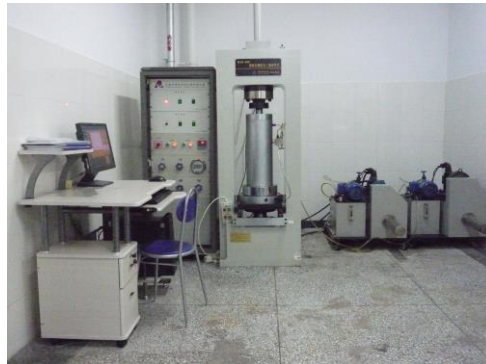
Figure 1. RLW-500 Rock Triaxial Apparatus for the Test
