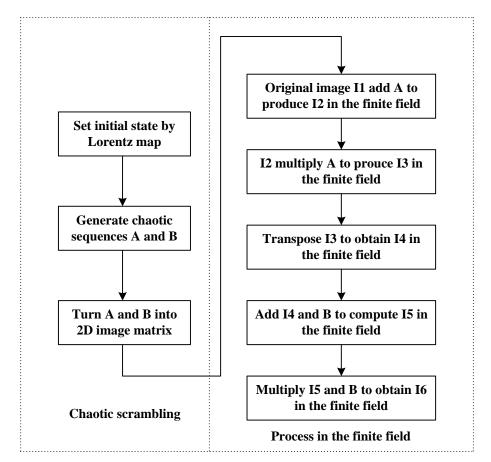
**Figure 1. Encryption Principle and Encryption Process**
