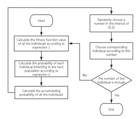
Figure 4. Flow Chart of Roulette Algorithm
