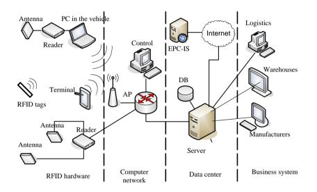
Figure 3. System Hardware Deployment Architecture
