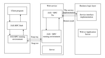
Figure 5. Principle of Web Services under J2EE Platform
