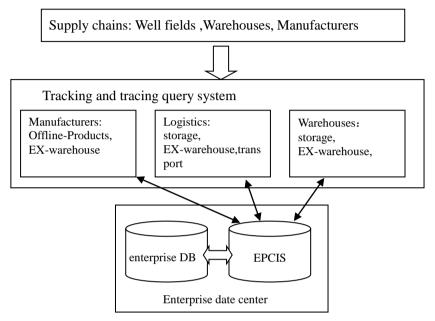
Figure 8. Tracking & Tracing Module Architecture Chart
