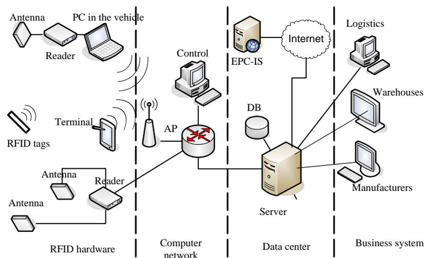
Figure 3. System Hardware Deployment Architecture
