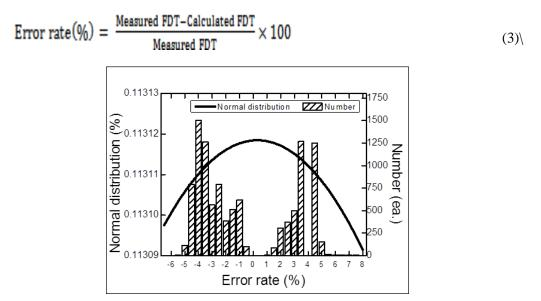
Figure 6. Normal Distribution on Error Factor Ratio of Calculated FDT and Measured FDT
