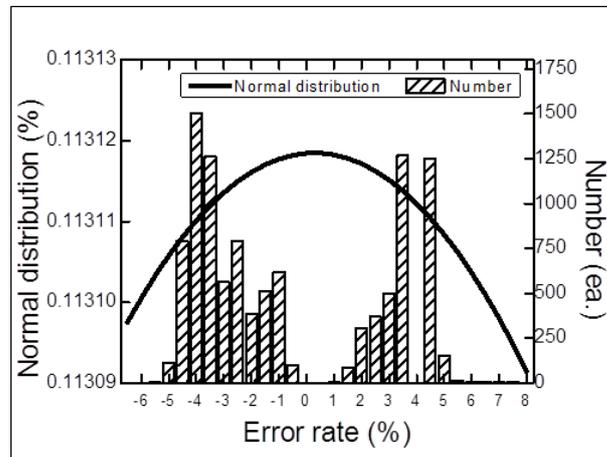
**Figure 6. Normal Distribution on Error Factor Ratio of Calculated FDT and Measured FDT**
