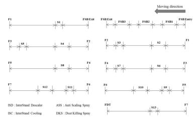
Figure 1. Layout of Finishing Mill Process
