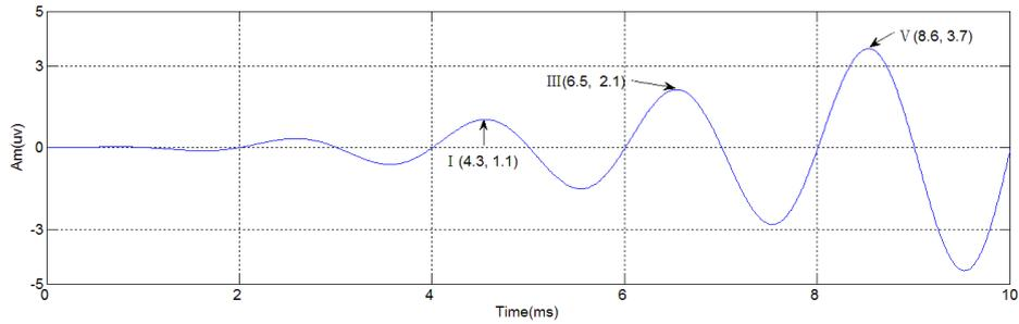
**Figure 2. Standard BAEP Signal Waveform**
