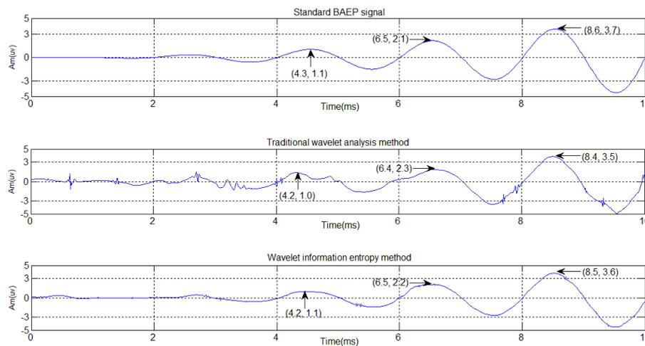
**Figure 4. Waveform of the Signal When SNR Is Equal to -2**
