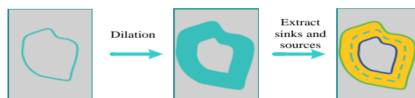
Figure 1. Extract Inner and Outer Contour of the CN using Dilation
