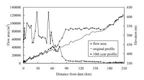
Figure 4. Delta Profile of the 10<sup>th</sup> Year and Flow Area Distribution (Flood Season)
