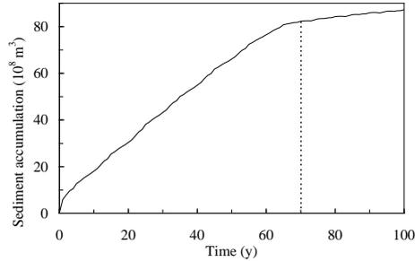
**Figure 1. Timewise Pattern of Sediment Accumulation in Reservoir**
