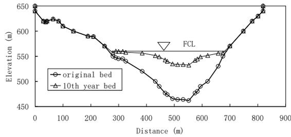
**Figure 16. Cross-section Evolution of Topset Section**
