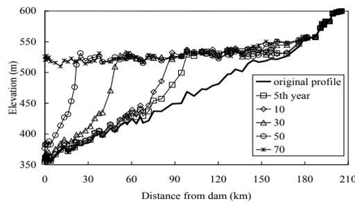
**Figure 2. Delta Profiles of Xi Luodu Reservoir in the First Stage**
