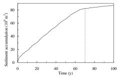
Figure 1. Timewise Pattern of Sediment Accumulation in Reservoir
