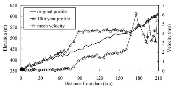
**Figure 3. Delta Profile of the 10<sup>th</sup> Year and Velocity Distribution (Flood Season)**
