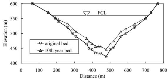
**Figure 10. Cross-section Deformation of the Foreset Section in the 10<sup>th</sup> Year**
