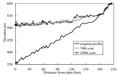
Figure 12. Delta Profiles of the Second Stage
