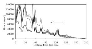
Figure 8. Flow area Distribution in Different Year (Non-flood Season) (The Arrow Direction Represents the 10<sup>th</sup>-70<sup>th</sup> Year)
