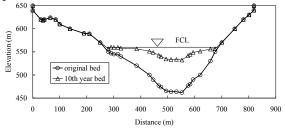
Figure 9. Cross-section Deformation of the Topset Section in the 10<sup>th</sup> Year
