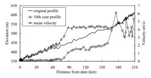
Figure 3. Delta Profile of the 10<sup>th</sup> Year and Velocity Distribution (Flood Season)
