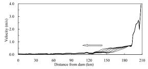
Figure 7. Velocity Distribution in Different Year (Non-flood Season) (The Arrow Direction Represents the 10<sup>th</sup>-70<sup>th</sup> year)
