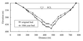
Figure 10. Cross-section Deformation of the Foreset Section in the 10<sup>th</sup> Year
