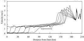
Figure 5. Velocity Distribution in Different Year (Flood Season) (The Arrow Direction Represents the 10<sup>th</sup>-70<sup>th</sup> Year)
