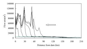
Figure 6. Flow Area Distribution in Different Year (Flood Season) (The Arrow Direction Represents the 10<sup>th</sup>-70<sup>th</sup> Year)
