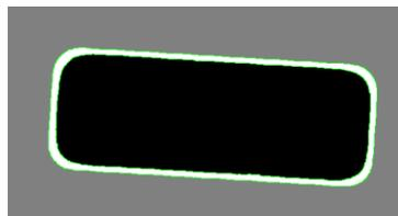
**Figure 7. Target Area of upper Surface of Magnetic Sheet Segmented by Maximum Entropy Method**
