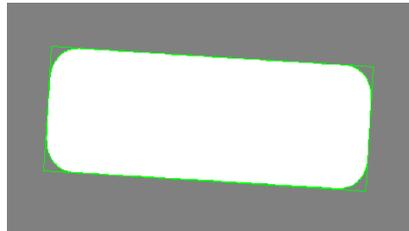
**Figure 2. Upper Surface of Magnetic Sheet after Binary Image Segmentation**
