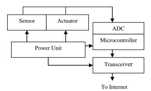
Figure 1. Sensor Node Architecture
