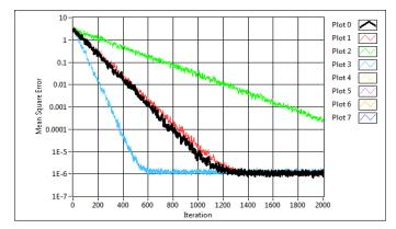
Figure 13. Learning Curve of LMS for different step sizes
