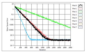
Figure 16. Comparison of VSS Algorithm with SLMS, LMS and NLMS Algorithm
