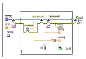
Figure 2. Block Diagram of Design of Adaptive IIR Filter using LMS Algorithm
