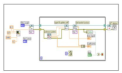
Figure 11. Block Diagram of VSS-LMS Algorithm
