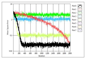
Figure 15. Learning Curve for Sign LMS Algorithm for Different Step Size
