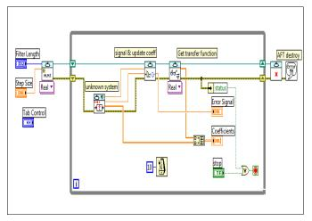
Figure 5. Block Diagram of Design of Adaptive IIR Filter using NLMS Algorithm
