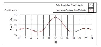
Figure 10. Adaptive IIR Filter output using Sign LMS algorithm
