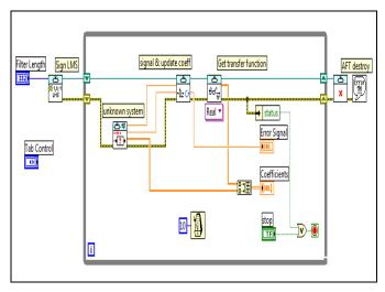
Figure 8. Block Diagram of SLMS Algorithm
