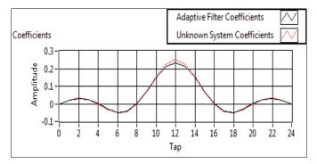
Figure 4. Adaptive IIR Filter output using LMS Algorithm
