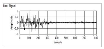
Figure 9. Error Signal using Sign LMS algorithm
