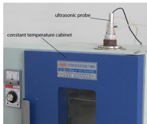
Figure 9. The Assembly Diagram of Ultrasonic Sensor in the Constant Temperature Cabinet
