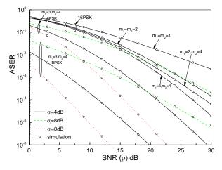
Figure 3. ASER of MPSK for the Dual-Hop Fixed Gain System versus the Un-Faded SNR (P)
