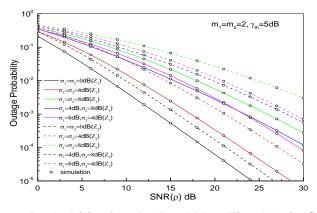
Figure 2. Outage Probability for the Dual-Hop Fixed Gain System versus the Un-Faded SNR (P) Under Different Shadowing Fading Parameters
