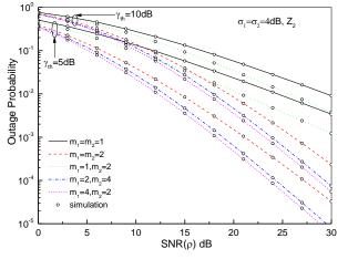
Figure 1. Outage Probability for the Dual-Hop Fixed Gain System versus the Un-Faded SNR (P) Under Different Multipath Fading Parameters
