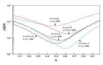
Figure 4. ABER Of BPSK For The Dual-Hop Fixed Gain System Versus D<sub>1</sub>
