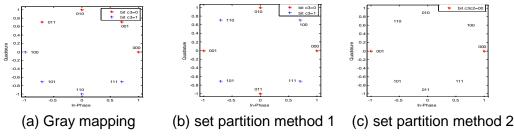
Figure 3. 8PSK Mapping Method
