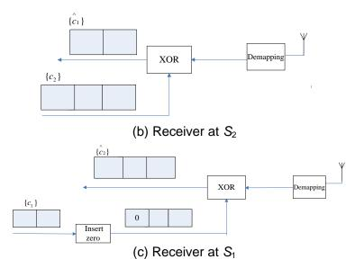
Figure 2. Transmitter and Receivers Diagrams in BRC Phase
