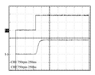
Figure 18. Ch1: Speed Response Sign Ch2: Speed Given Sign
