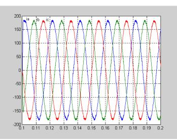
Figure 13. The Simulation Waveform of 3-Phase Output Currents
