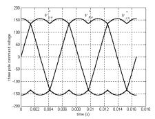
Figure 8. Waveform of Three Pole Command Voltages of Naturally Sampled
