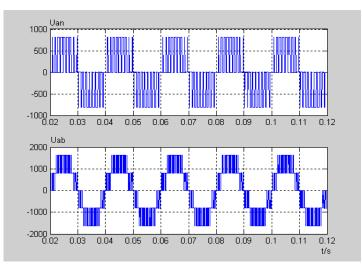
Figure 12. The Simulation Waveform of Phase Voltage Ua and Line Voltage Uab in Switch Mode
