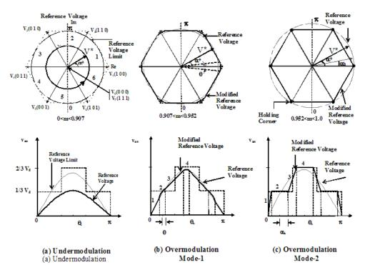
Figure 6. Voltage Trajectories in Undermodulation and Overmodulation Regions and the Corresponding Phase Voltage
