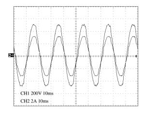
Figure 15. Single Input Voltage and Current Wave in Rectifier
