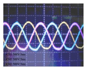
Figure 17. Three Phase Output Voltage in Inverter
