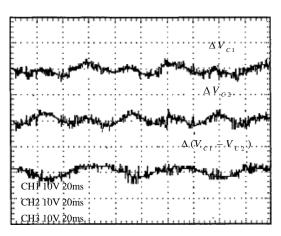
Figure 16. Voltage Error between Dual Dc Capacitor
