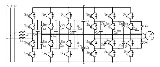
Figure 1. The Topology of Hybrid Clamp Three Level Three Phase Converter
