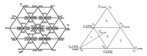
Figure 9. Space Voltage Vectors of Hybrid Clamp Topology Figure 10. Space Voltage Vectors of Hybrid Clamp Topology
