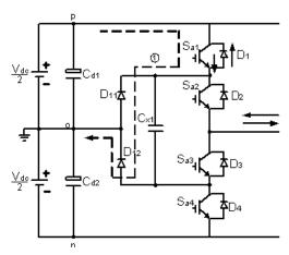
**Figure 2. P Vector Current Circuit**
