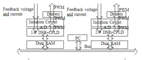
Figure 14. Control System of Dual Pwm Hybrid Clamp Topology
