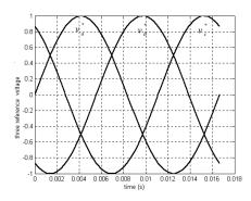
Figure 7. Waveform of Three Reference Voltages of Naturally Sampled SPWM
