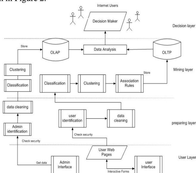
**Figure 2. Shows the Proposed Four Bottom-Up Layers**
