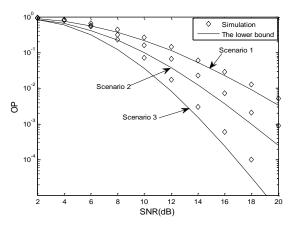
Figure 1. The OP Performance Over N-Nakagami Fading Channels
