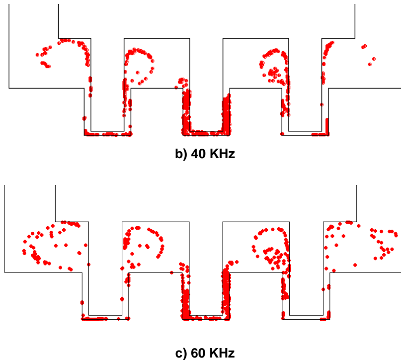
Figure 3. Debris Distribution of Flow Field Under Different Frequency of Ultrasonic Vibration after Completing 500 Microseconds Ultrasonic Vibration
