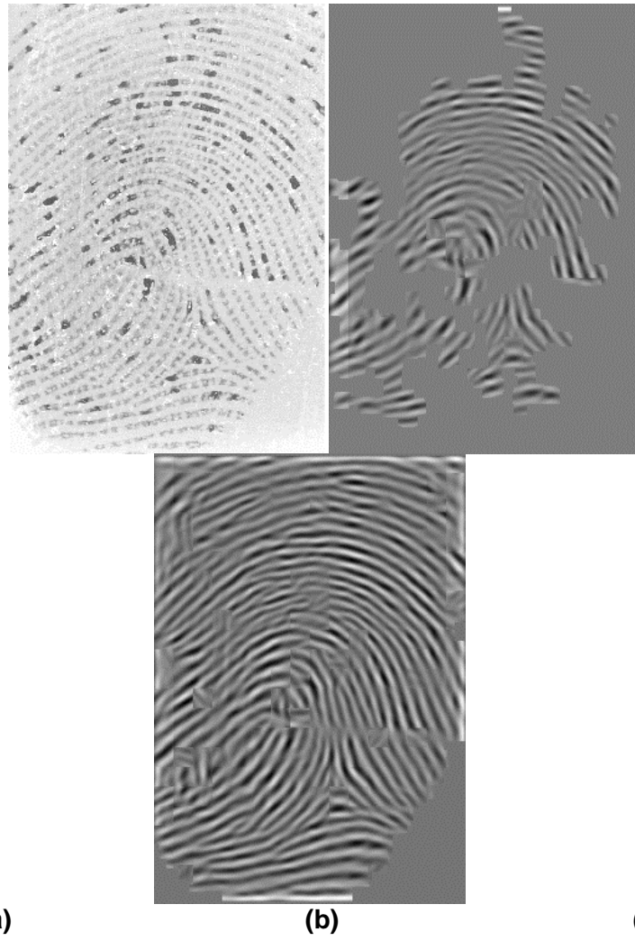
Figure 9. a) Bad Quality Image, b) Gabor Enhancement, c) Proposed Method Result
