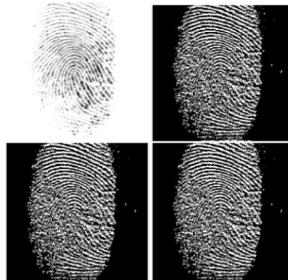
Figure 1. Fingerprint Image and Wavelet Decomposition
