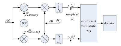
Figure 1. Structure of PN Code Acquisition System
