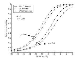
Figure 2. Detection Probabilities of the Conventional SS Detector, the NAI-LO Detector and the Proposed Schemes for Different *rs* and  $\rho$  when  $P_{fa} = 10^{-2}$  and M = 50 in Multiplicative and Weakly Dependent Non-Gaussian Noises
