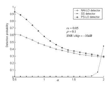
Figure 5. Detection Probabilities of the Detectors as a Function of  $\alpha$  for Some Values of  $\rho$ , *rs* and SNR/chip when  $P_{ia} = 10^{-2}$  and M = 50
