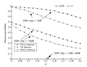
Figure 3. Detection Probabilities Plotted as a Function of  $\rho$  for some Values of SNR/chip and *rs* when  $P_{fa} = 10^{-2}$  and M = 50 in Multiplicative and Weakly Dependent Non-Gaussian Noises for  $\alpha = 1$
