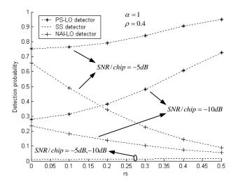
Figure 4. Detection Probabilities Plotted as a Function of *rs* for Some Values of SNR/chip and  $\rho$  when  $P_{fa} = 10^{-2}$  and M = 50 in Multiplicative and Weakly Dependent Non-Gaussian Noises for  $\alpha = 1$
