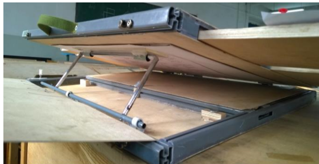
Figure 6. Load-bearing of the Supporting Pole
