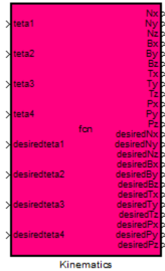
Figure 7. Kinematics Embedded MATLAB Function
