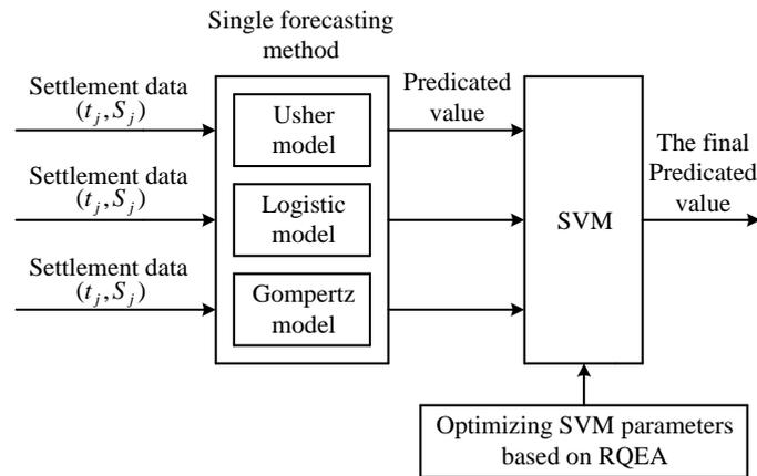
**Figure 1 Combined forecasting model based on RQEA and SVN**
