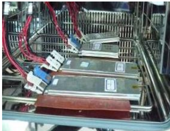
Figure 1. Batteries for Test
