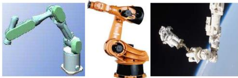
Figure 3. Examples of Serial Manipulators with Six DoF in a Kinematic Chain
