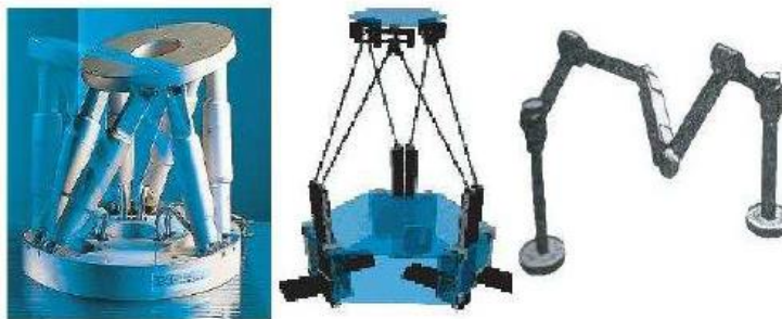
Figure 4. Typical Parallel Manipulators
