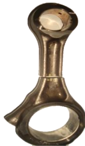
Figure 2. Sample 'A1' Prototype Failed at Big End
