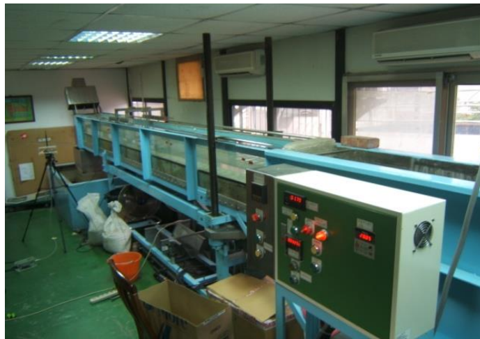
Figure 7. Water Circulation Channel
