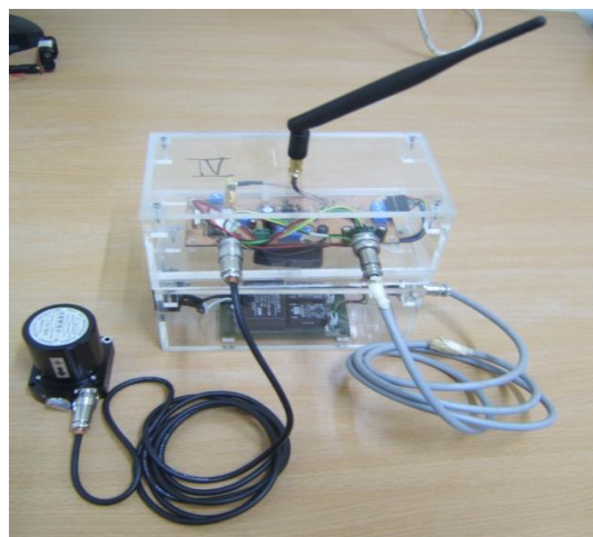
Figure 4. The Installation of Sensor and Infrastructure Node
