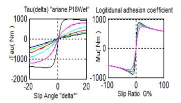
Figure 4. Relationships between Longitudinal and Side Adhesion Coefficient using the Magic Formula
