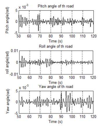
Figure 5. Plan Angles of the tire/road Surface Contact
