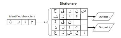
Figure 22. Classification of a Word with Two Possibilities
