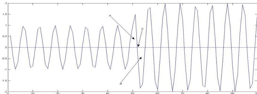
**Figure 4. Discontinuous Point Makes the Fourier Integral of the Signal Appear Slow Decay**
