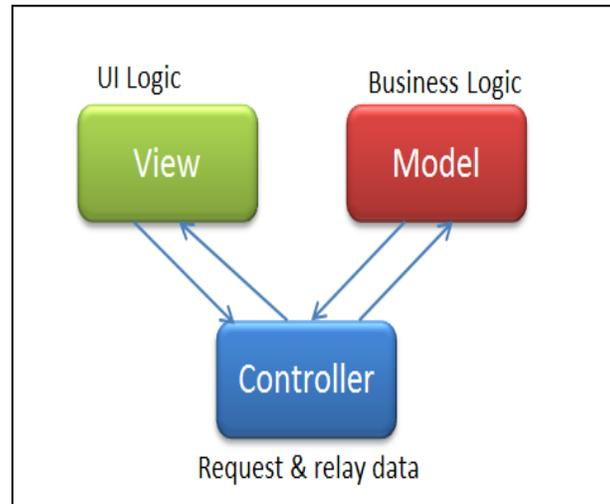
**Figure 1. MVC Components**
